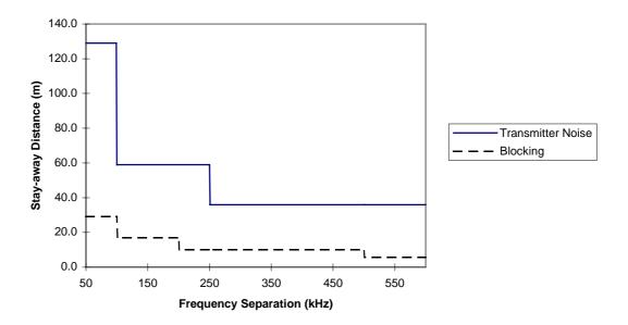
Figure 25: Stay away distance to ensure effects of blocking Tx or wideband Tx interferer are at negligible level
