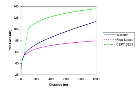
Figure C.1: Calculated path loss for the three propagation models h<sub>1</sub>=1.5m, h<sub>2</sub>=2m
