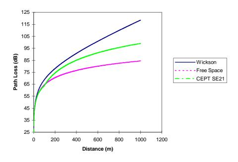
Figure C.3: Calculated path loss for the three propagation models  $h_1 = 10 \text{ m}$ ,  $h_2 = 30 \text{ m}$
