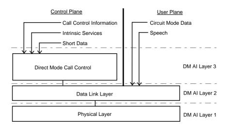
The DM MS-MS protocol stack for MS-MS operation is shown in figure 13.
